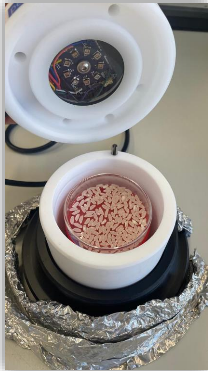
3 g of infested rice treated with UV-C 280nm
