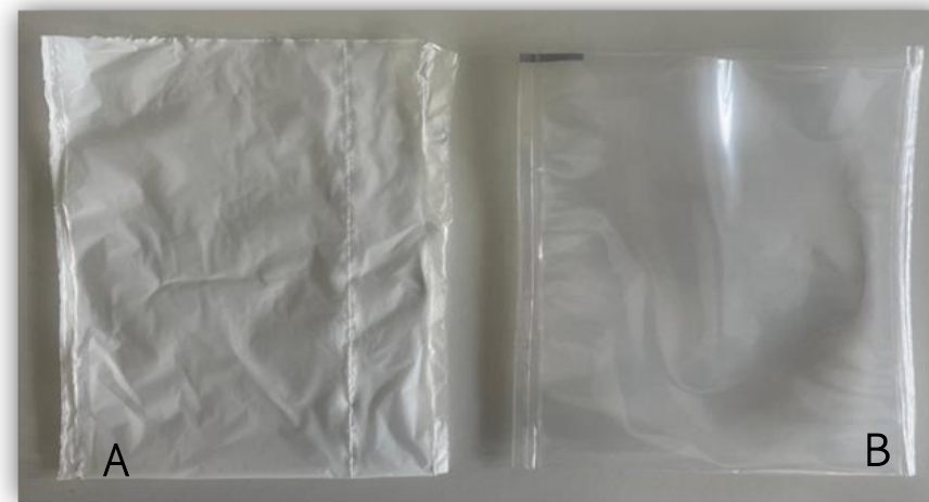
A – biodegradable packaging; Mater-Bi (EN 13432 standard) B – traditional petrochemical plastic (BOPP with a 30 µm transparent layer and a 70 µm transparent PE layer)
